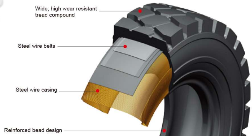
ALL-STEEL RADIAL INDUSTRIAL VEHICLE TIRE CROSS-SECTION DRAWING
